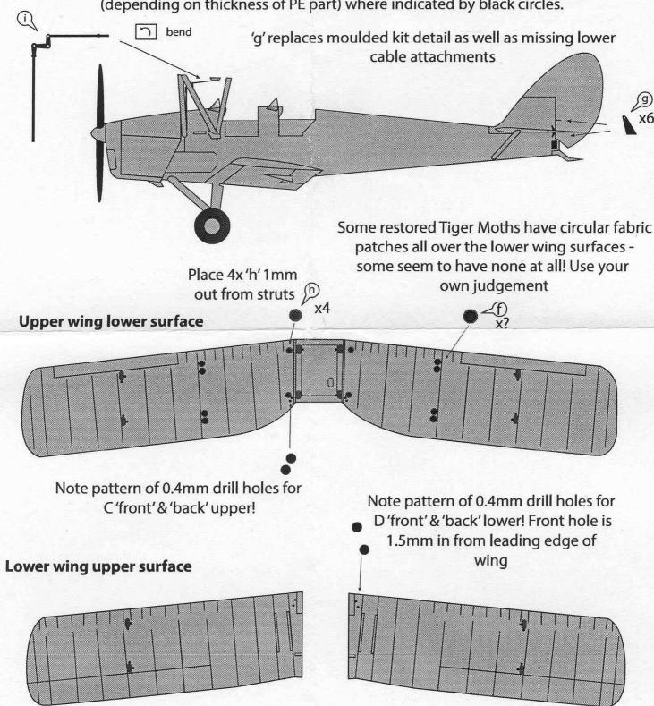
Note - PE Bracing wires follow Airfix kits alphabetical indicators and also diagram with the exception of 'A' upper which should be at base of upper forward struts
