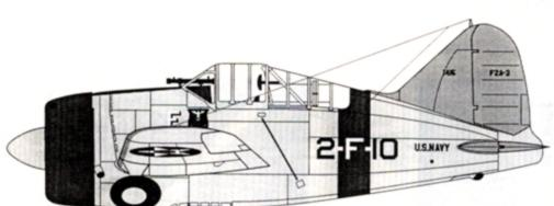
F2A-2 Buffalo, Bureau Number 1415, VF-2, USS Lexington, 1941. Overall aluminum lacquer finish with Orange Yellow upper wing surfaces carried around leading edge. Vertical and horizontal tail surfaces Lemon Yellow. Forward cowl, fuselage band, and upper wing chevrons glossy black. Antiglare panel flat black. Note modified antenna arrangement with mast removed and wire attached to upper wing.
