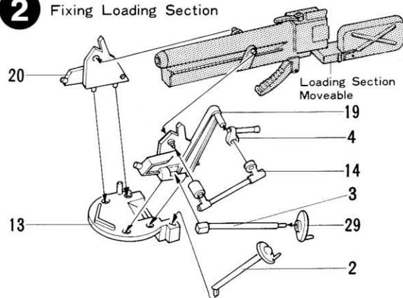
★When you fix parts 29 & 3, refer to the plans below and cement in position.
