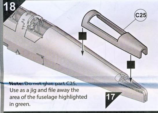
**Note:** Do not glue part C25. Use as a jig and file away the area of the fuselage highlighted in green.
