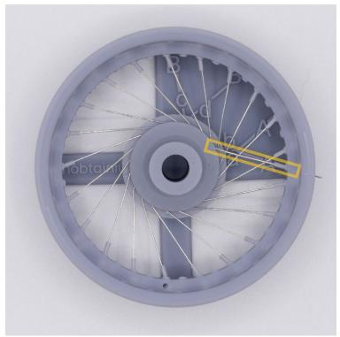
Continue as before, using CA on the Hub end only, inserting the nipples, but not fixing with CA yet. you should get to here
