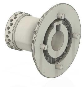
Ensure the rear face is flat, removing all print supports as necessary, but not the four pins above.
