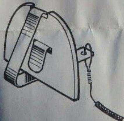
The two metal strips are battery terminals and these should be fitted to the two supports contained in Frog models with the word "SPIN" after the reference number. The folding of these terminals varies and further diagrams giving the correct shape will be found in the leaflet packed with each "SPIN" model. To use "SPIN-A-PROP" with other models you will have to make supports to suit your own requirements.
