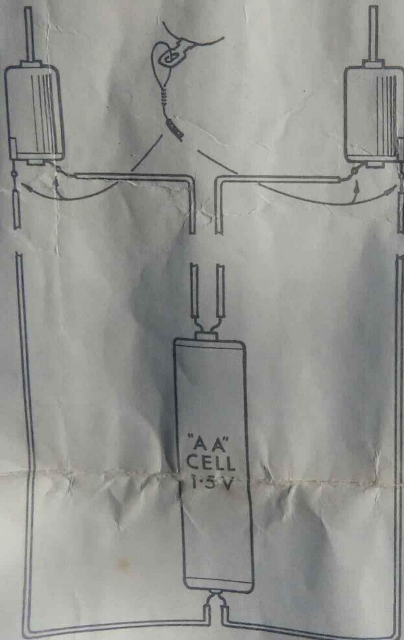
The wiring diagram shows the connections, within the model, between the motors and the battery.
