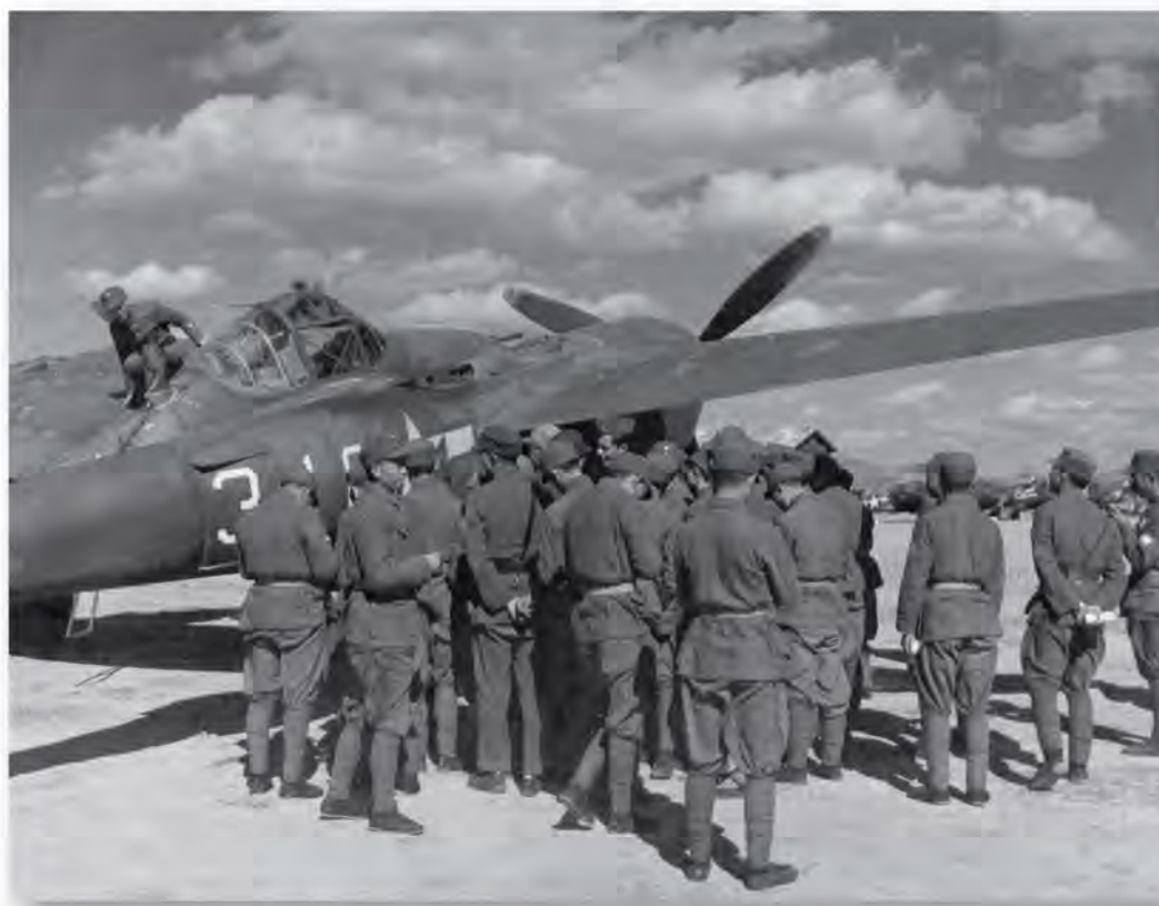
A curious group of Chinese soldiers inspect a 449th FS P-38 at Kunming. The Lightning was new to their part of the world, and undoubtedly attracted attention wherever it was seen. Note the three digit side number, the prominent ADF loop antenna and its mount aft of the cockpit, and how the crushed stone had already begun to scour the paint from the back side of the prop blades.
