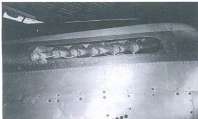
An example of the unshrouded exhaust is shown here. (Detail & Scale photo by Bert Kinzey)
