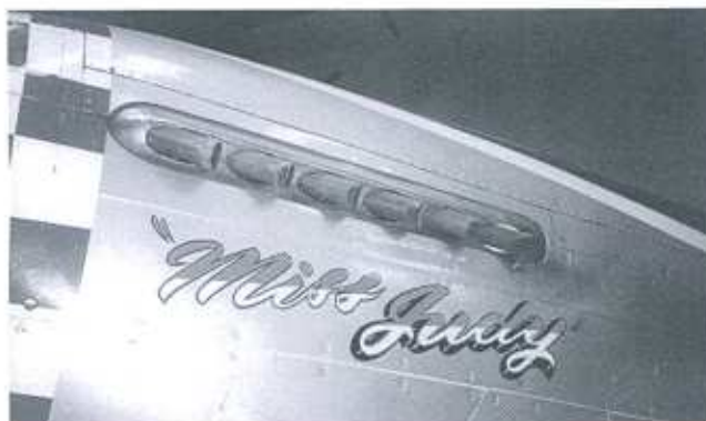
This is what the shrouded exhaust looks like. (Detail & Scale photo by Bert Kinzey)
