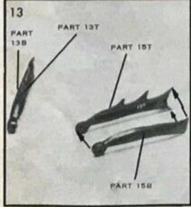
Glue parts 15T and 15B together. Do the same with 13T and 13B. Mark with pencil.
