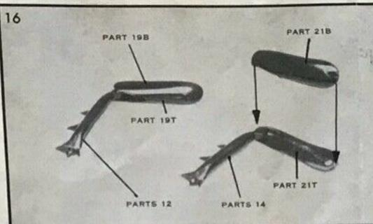
Place part 15 on the pivot pin of part 21T. Now glue part 21B to 21T. Assemble parts 13, 19B, and 19T in the same way. Mark the parts with your pencil.
