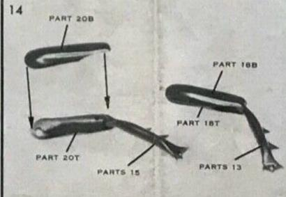
Place part 15 on the pivot pin of part 20T. Now cement 20B to the unit. Assemble part 18B 18T, and 13 in a like manner. Mark parts with a pencil.
