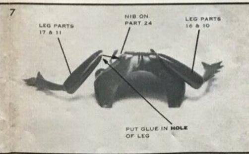
Place glue in the holes of the leg parts and attach them to the nib of part 24 as shown above.
