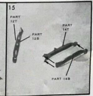
Glue part 14T to 14B as shown. Do the same with parts 12B and 12T as shown. Be sure to mark part numbers on the outside of the piece with a soft pencil.
