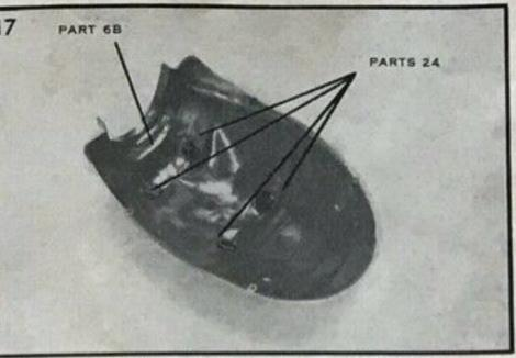
Place parts 24 through the holes in part 6B. Do not glue.
