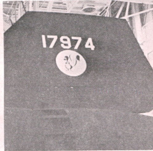
Outside surface of left fin and rudder. This is 17974 after major overhaul and repaint at Lockheed-Palmdale.
