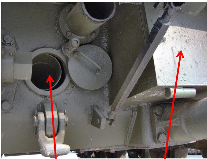
ENGINE HEATER EXHAUST HOLE, WITH COVER
